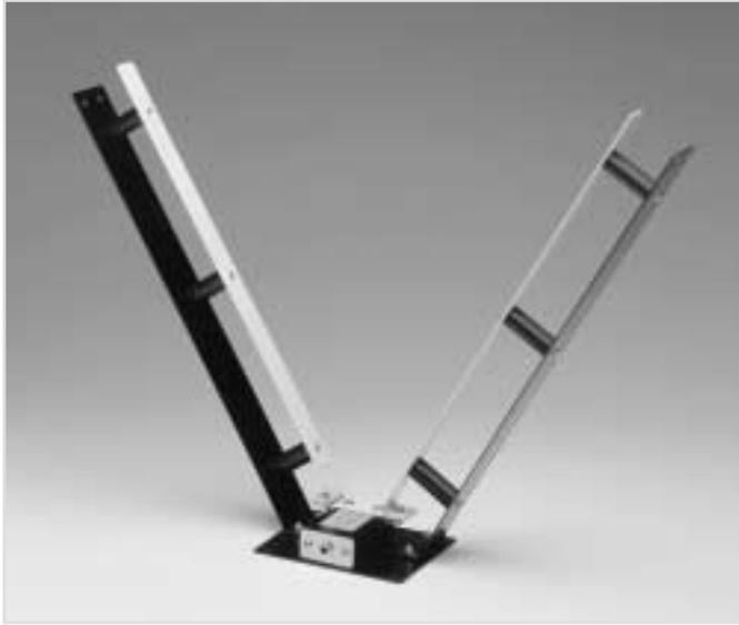
The length of your coupler cable will determine how far from the control unit you can position the antenna assembly, but a minimum distance of three feet (3' or 1 meter) is strongly suggested. This helps to ensure that the operator's body is not close enough to the antenna to affect the tuning. The standard cable length is eight feet (8' or 2.4 meters), and optional lengths of fifteen feet (15' or 4.6 meters) and twenty-five feet (25' or 7.62 meters) are readily available.
